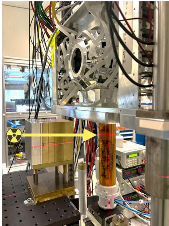
Figure 24. ^{11}\text{C} irradiation setup. Mouse fixed on the SIRMIO bed and positioned in front of the beamline, with the back facing the beam exit; the same configuration was used for both the
