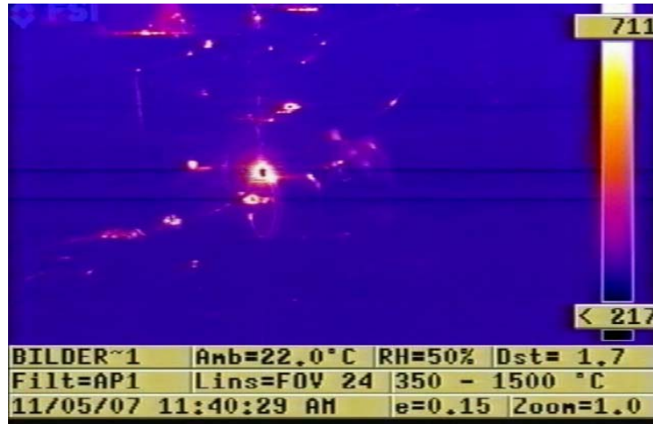
Figure 71: Absorption image of the thermal camera in the temperature range of 217°C to 711°C during the welding process.
