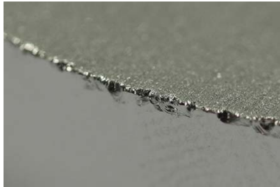
Figure 14: Example of edge chips.
