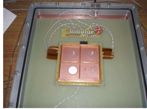
(a) A 2-GEM assembly under test in lab.
