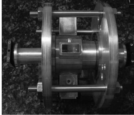
Figure 13: Photo of a prototype CBPM developed at SINAP in 2008. Taken from [52].
